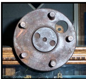
9 inch - 31 spline axle Counter sunk holes in the center indicate a 31 spline axle. 31 spline axles are uniform in diameter.
