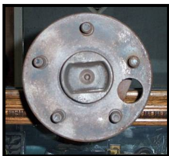
9 inch - 28 spline axle Note the concave oval area in the center of the axle flange. Early 28 spline axles are tapered.
