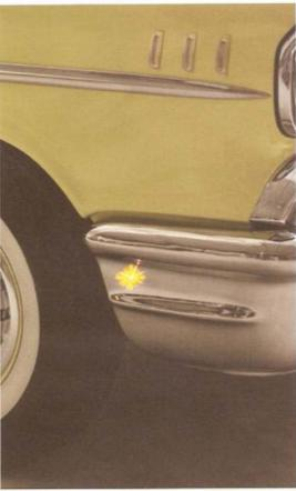
Visibolts® used as side marker lamps In stock bolt location. No drilling
