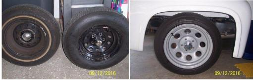
2 – P215/75R15 BF Goodrich T/A 8/32" tread, no cracks, no plugs, mounted on 8" x 15" Diamond Wheel 10 hole steel wheel - black. Wheel fits 5 x 4.75" bolt circle and has 4" back space with 3.25" center hole. Comes with generic chrome metal center cap. Asking \$75/OBO for pair.
