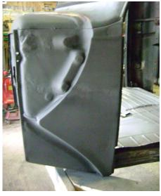
If one of the photos looks familiar you might have a Taurus, I used the structure under the hood of a Taurus for the main support. I had access to plenty of free sheet metal since I worked at Kayser Ford and could raid the metal dumpster whenever I needed. One of my best purchases was that of a bead roller as you can see in the last photo, The floor & fire wall got massive amounts of rolled beads for strength. I even made some different dies for the roller on my lathe.
