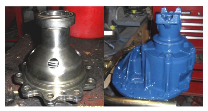
The first photo is of the locker before I replaced the bearings & installed the ring gear & the second is of the finished unit (painted Ford blue of course). I picked up the bench mounted holder from Summit Racing for about \$50.00 & it sure worked nice.
