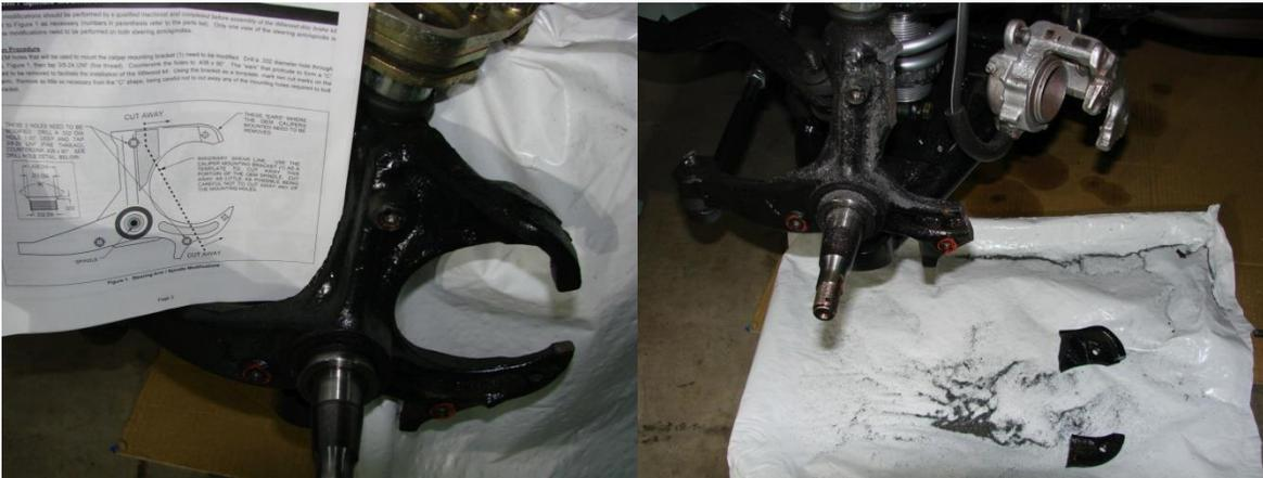
By drilling and tapping two former dust shield bolt holes, they now became threaded holes for the new caliper bracket. The drill bit used was a .332" (Q) drill, and the tap was a 3/8-24. The top hole was drilled to 1" deep and the bottom hole drilled through. Once tapped, the holes were flushed with brake cleaner to remove all cuttings.
