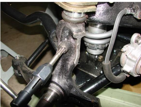
Once all the cutting, drilling and tapping was done, I cleaned up the cut areas with a grinder, sprayed everything off with brake cleaner, and applied some paint. Once the paint was dry, it was time to mount the caliper bracket, and install the hub on the spindle. The axle nut secures the outer bearing and washer. Once adjusted to the OEM specs for drag on the bearings, a new cotter pin was installed to prevent the axle nut from turning, and the dust cover was screwed into place.
