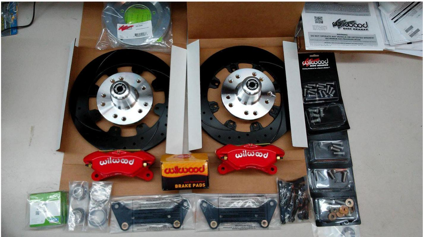
The hub and rotor pieces were assembled, prior to installation on my truck. All bolts had Red Locktite applied before threading in and getting torqued to 40ft/lb. The hub is set up with a dual bolt pattern. I'm using the 5 X 4.75" GM pattern. 5 X 4.5" is the other option.
