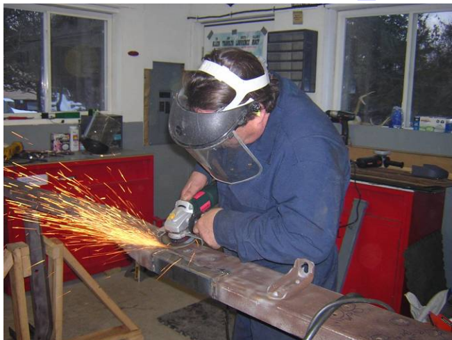
Dean Malin grinds the welds smooth while Chuck Blanchard welds the holes. Paul Hilgers waits to grind welds.
