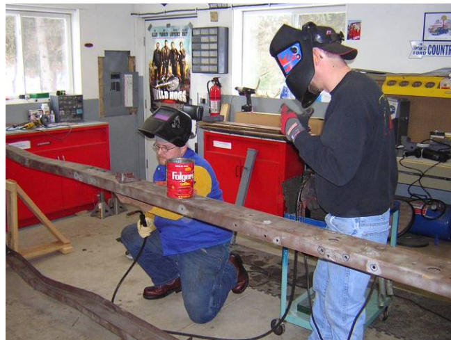
Dean Malin grinds the welds smooth while Chuck Blanchard welds the holes. Paul Hilgers waits to grind welds.
