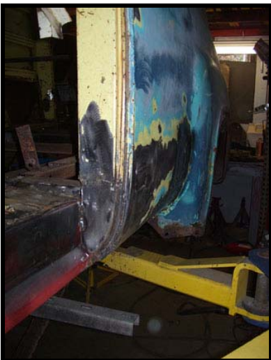
Metal patching- Drivers door and back. (12/10)
