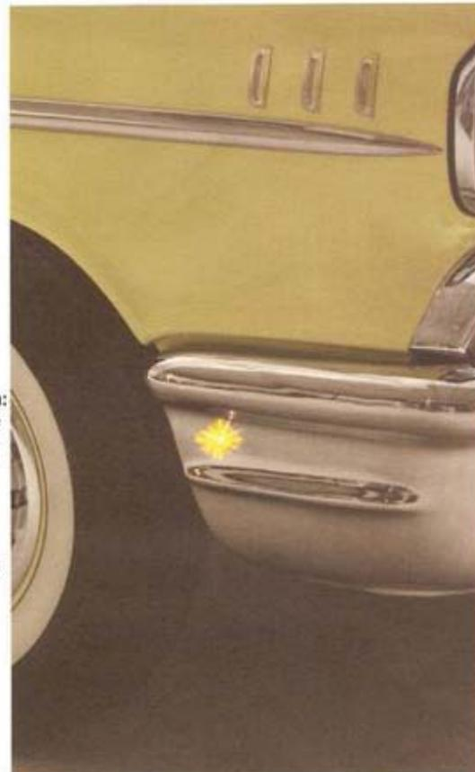
**Visibolts® used as side marker lamps**
